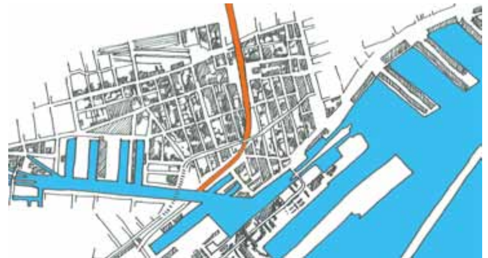
Figure 2.47: An elevated railway crosses Griffintown to connect the Victoria Bridge to the central station.
